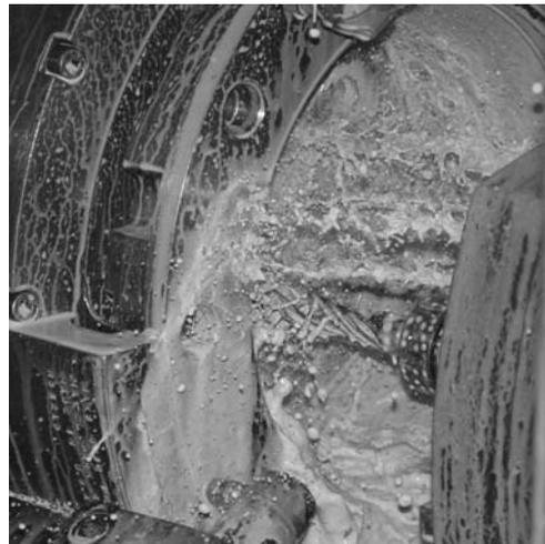
*Developing fluid in a lathe machine*
