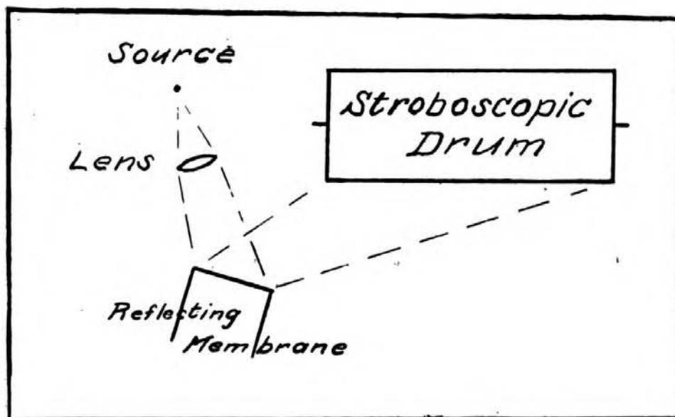
FIG. 23—Lighting Scheme in New Tonoscope.
