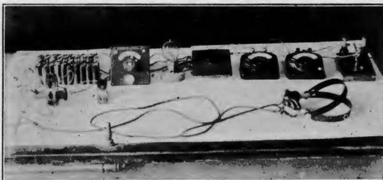
The frequency of the current was found to increase by decreasing the capacity of the condenser, decreasing the inductance  $L_2$ , increasing the inductance  $L_1$  and as the filament current approaches the most favorable value for the filament.
