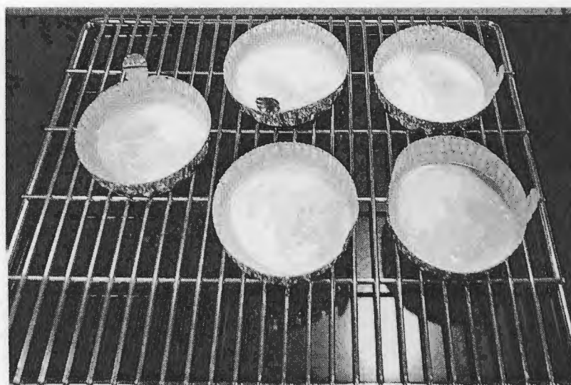
Figure 2. Aluminum Dishes Ready to Place in the Oven
