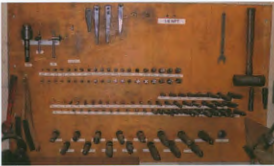
Figure 5. Photograph of the Machining Area board providing designated spots and labels for taps, drills, and other necessary items.
