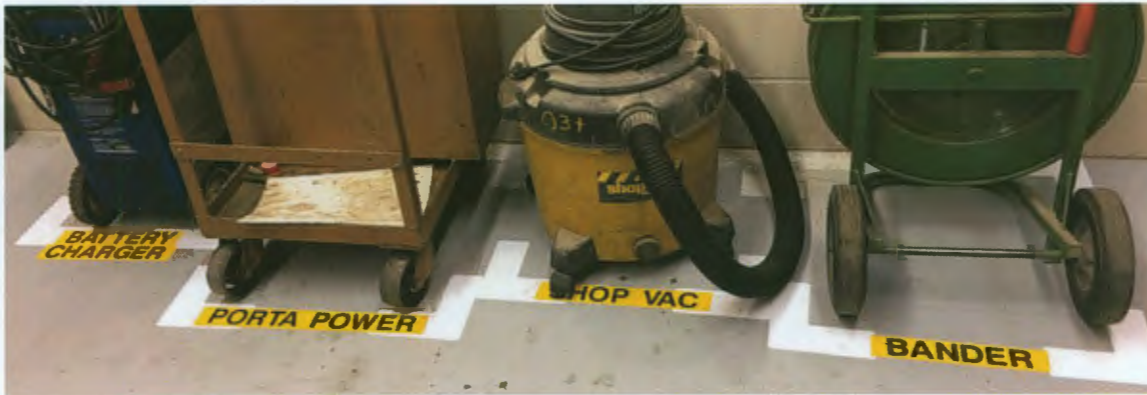
Figure 8. Photograph showing floor markings and labels to give items a “home.”
