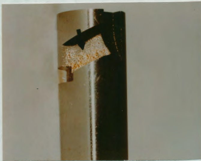
Figure 7. A photograph showing the deposits in the helix of a typical fuel injection pump plunger.
