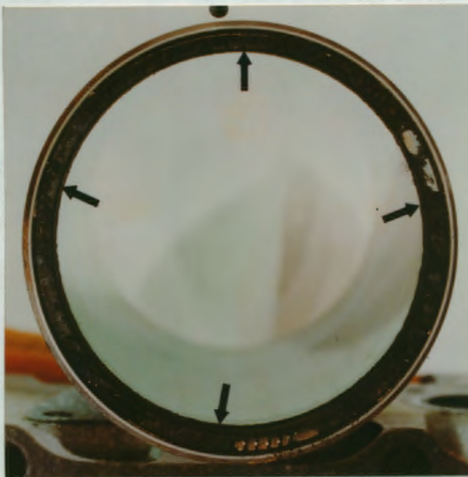
Figure 4. A photograph showing the carbon deposits on the top flange of a typical cylinder liner.
