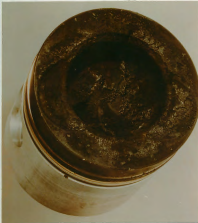
Figure 1. A photograph showing excessive carbon deposits on the head and in the combustion bowl of a typical piston.
