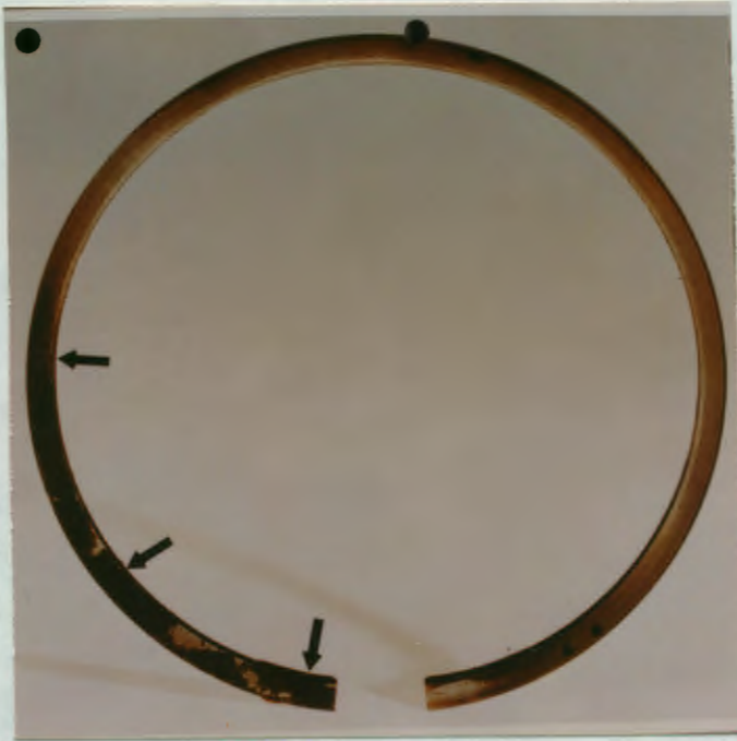
Figure 3. A photograph showing the carbon deposits on the top side of a typical number two piston compression ring.
