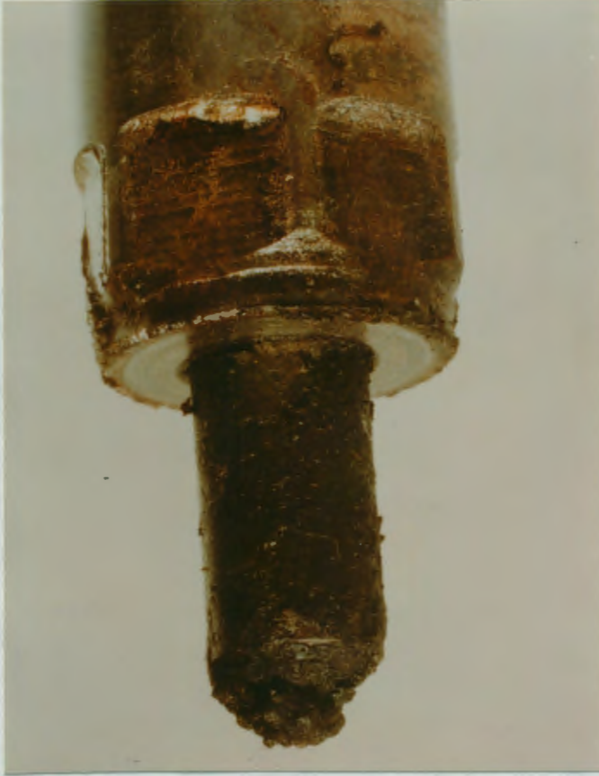
Figure 6. A photograph showing the excessive carbon deposits on the tip of a typical fuel injector.
