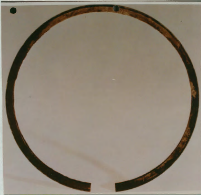
Figure 2. A photograph showing the carbon deposits on the top side of a typical number one piston compression ring.
