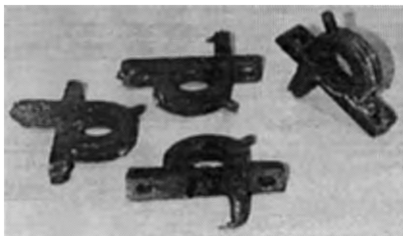
Fig. 4 LS Vac Castings (2365°F, 10"Hg)
