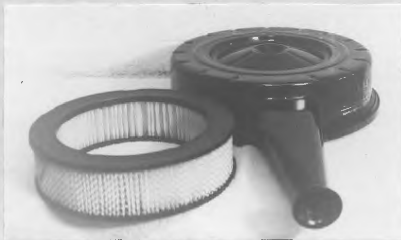
Figure 11. General Motors Air Cleaner Housing With Large Filter Element
