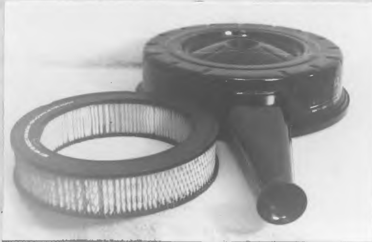
Figure 13. General Motors Air Cleaner Housing With Small Filter Element
