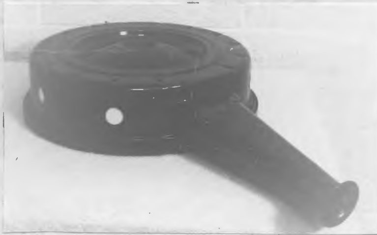
Figure 12. General Motors Air Cleaner Housing With Breather Holes
