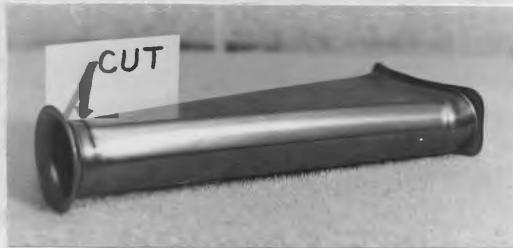
Figure 9. General Motors Test Snorkel With Flare Removed
