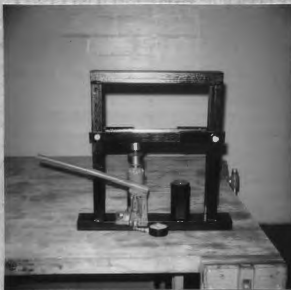
Figure 9. Compression tester constructed in the laboratory.
