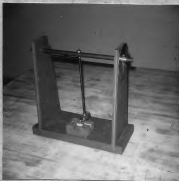
Figure 12. Laboratory build impact strength testing apparatus.
