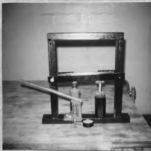
Figure 5. A tensile tester constructed in the laboratory.
