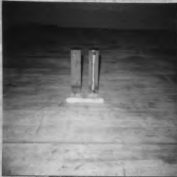
Figure 4. Steel injection mold in dog bone shape for producing tensile test specimens.
