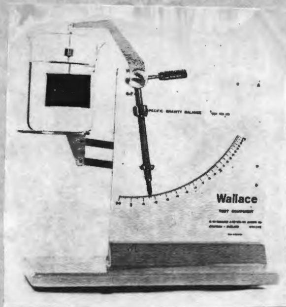
Figure 13. A direct reading specific gravity balance (Baird, 1971, p. 73)
