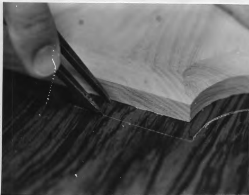
Figure 10. Scoring Along an Irregular Surface with a Divider
