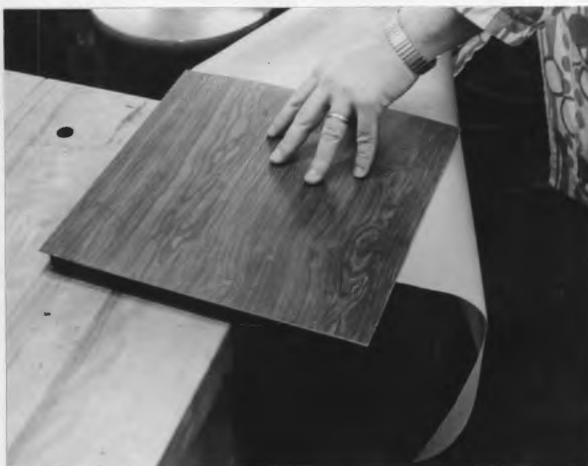
Figure 16. Slip-sheet Method of Aligning Laminate over Substrate
