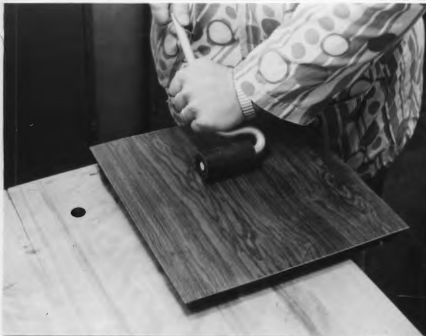
Figure 17. Applying Pressure with the Hand Roller
