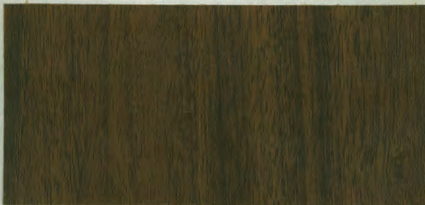
Figure 1. Example of Vinyl Film .006 inch Thick (Phillips 66 Film Division).
