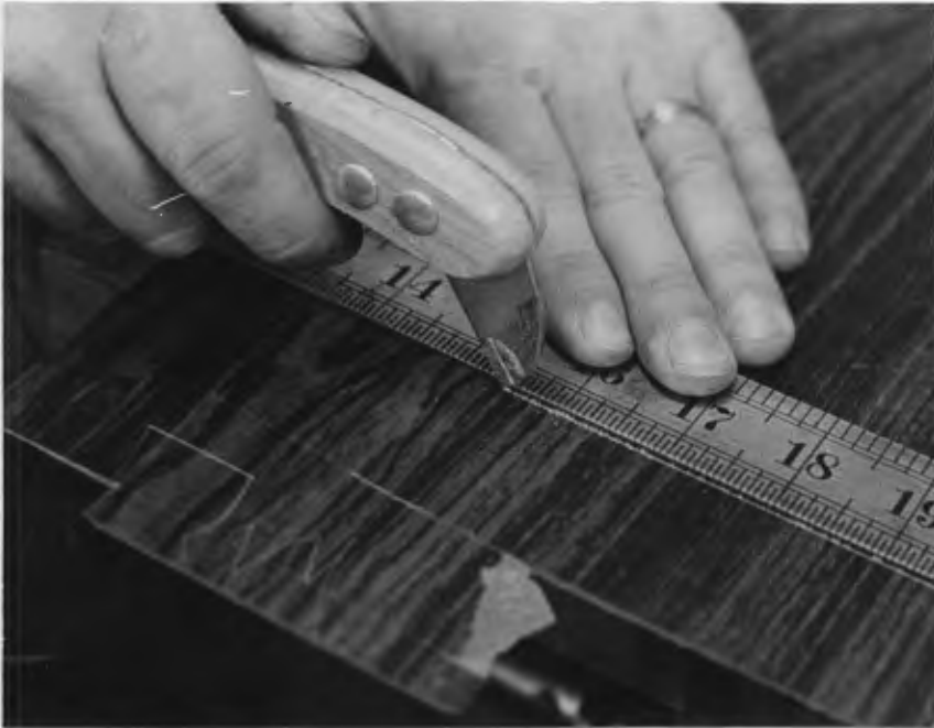
Figure 9. Scoring with a Carbide-tipped Score Awl
