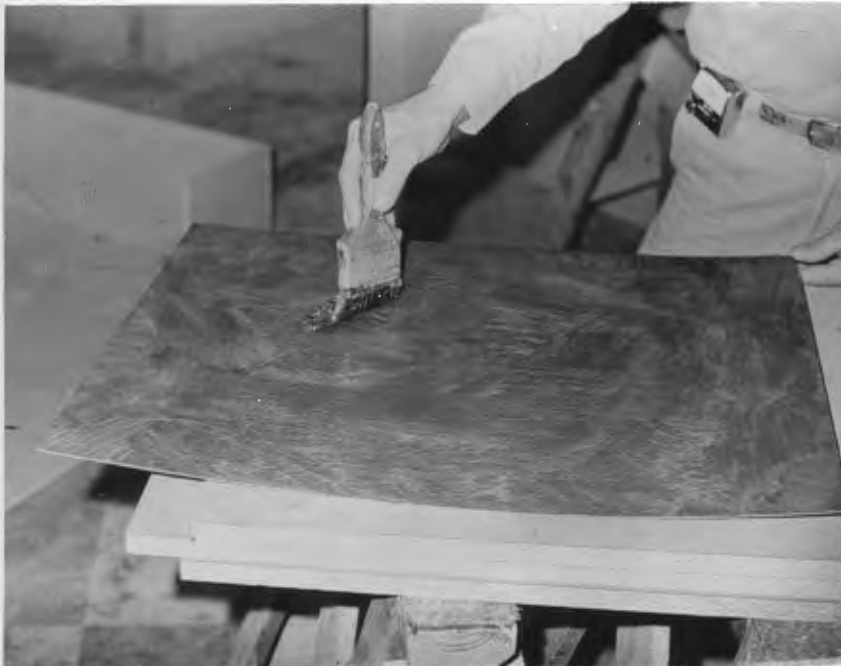
Figure 11. Applying Contact Cement with a Brush
