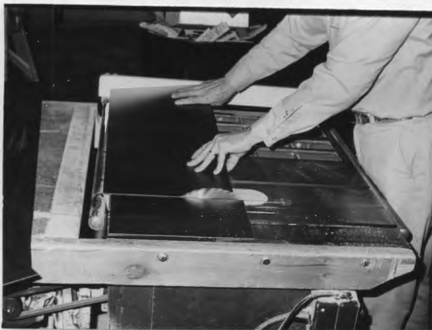
Figure 6. Cutting Plastic Laminate
