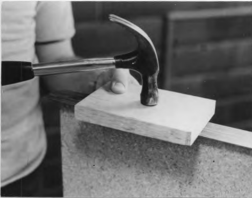
Figure 14. Applying Pressure to Edges with a Block of Wood
