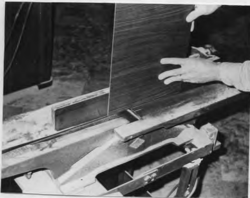
Figure 7. Jointing Plastic Laminate
