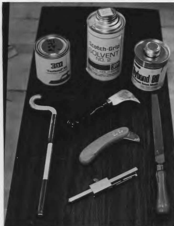
Figure 8. Materials and Tools for Plastic Laminate Application
