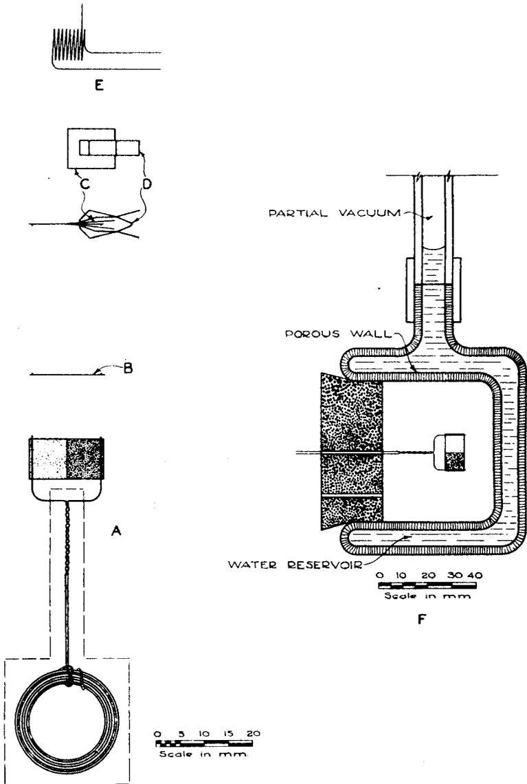
Fig. 1. Bismuth antimony thermojunction for measuring relative humidity.
