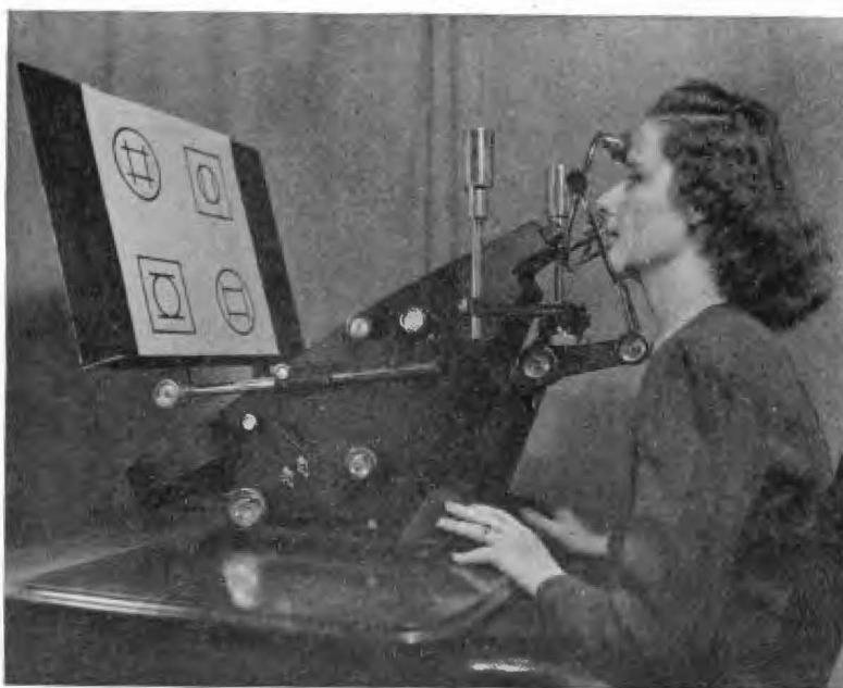
Fig. 2. A Bidimensional Eye-movement Camera and Exposure Card; the monofilm Camera was invented and developed by the author of this study. Patent rights have been issued by the U. S. A. Patent Office.
