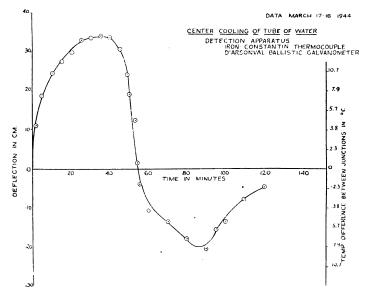
ginning with tap water, the warm water rises. As the temperature drops due to the ice pack, the top and bottom temperatures come to the same temperature. At this point the thermo-electric current reverses, indicating that the top junction is colder. For demonstration purposes, it is sufficient to observe deflections, the galvanometer and couple could be calibrated in degrees difference of temperature. These data were taken by Miss Gerry Ross, a major student in the Department.
