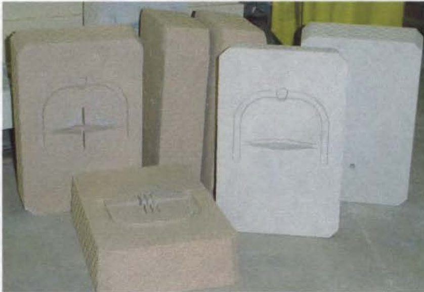
Figure 19. Experimental molds made out of no-bake sand
