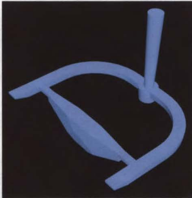
Figure 16. Test casting with attached gating system (the pressurized gating system with ratios 2:3:1 was used)
