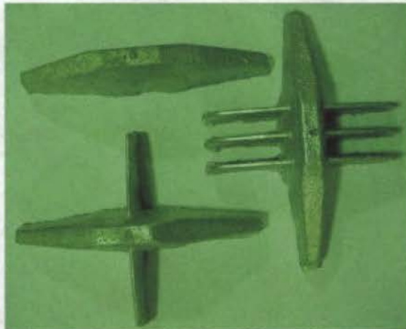
Figure 21. Experimental castings (gating components are removed)
