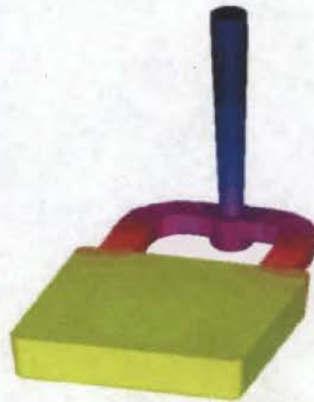
Figure 7. Test casting used for the establishing of the baseline data (color shows temperature distribution after completion of the solidification)
