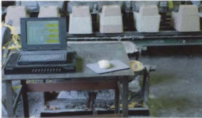
Figure 20. Data acquisition system in front of the pouring deck
