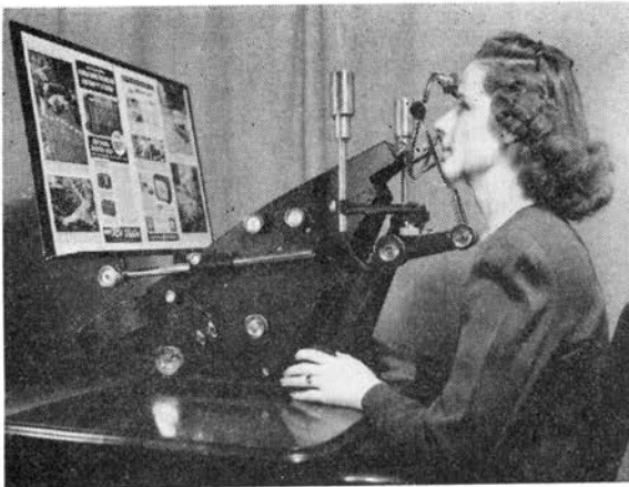
Fig. 4 A bidimensional mono-film camera, developed by the author.
