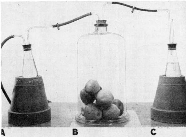
Fig. 4. Apparatus Used to Collect and Identify the Volatile Compounds Arising From Apple Fruits. A. Collecting Flask Containing Test Reagent and Tube Leading to Aspirator. B. Sealed Bell Jar with Apple Fruits. C. Scrubbing Flask with Tube to Atmosphere.
