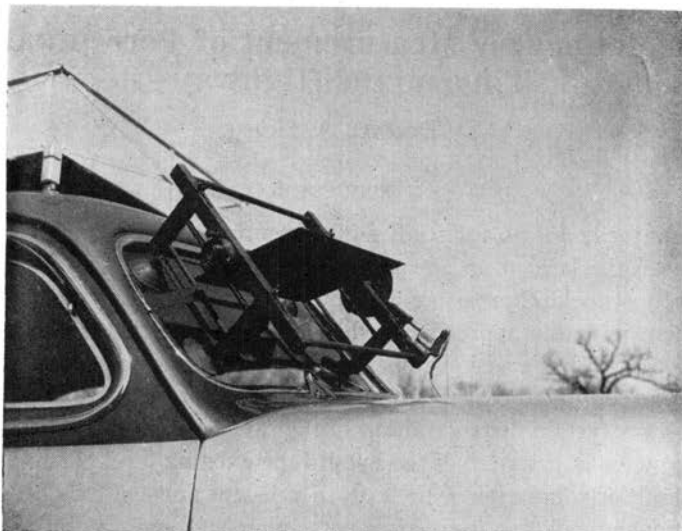
Figure I. Tachistoscopic and short time exposure apparatus mounted on a car. On the left side is the coil spring, center the aluminum shutter, and on the right the solenoid, lever, and ratchet wheel.
