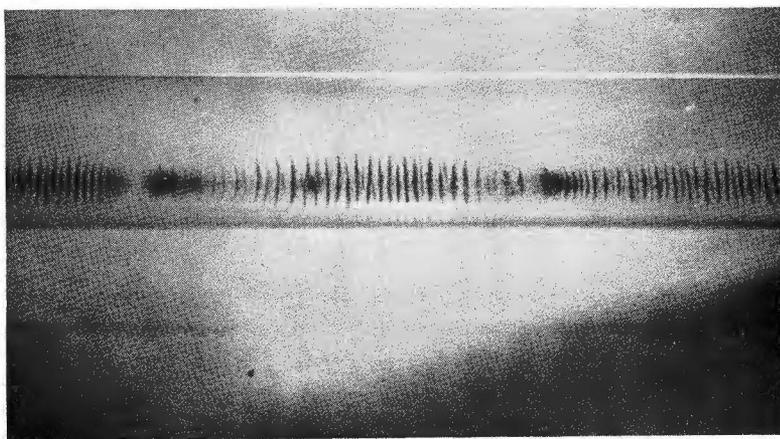
Figure 2. This shows a portion of a cork dust pattern in a Kundt tube. The photograph was taken after the source of sound had been turned off. The ridges do not appear as sharp and straight as they actually do when the sound is turned on.
