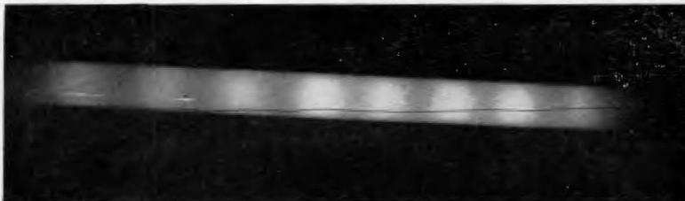
Figure 1. This is a photograph of a striation pattern in a 2-foot fluorescent tube. Although the ends are not visible the pattern extends the entire length of the tube. The black line crossing the pattern is a portion of one of the Lecher wires.
