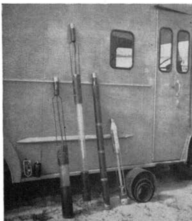
Figure 7. "Down-the-hole instruments used in electrical well logging, including flow meter, flow meter housing, fluid conductivity electrode, electric logging electrode, and caliper. Temperature electrode not shown.
