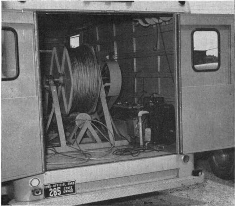
Figure 6. Four conductor cable, mounting and 110-volt a.c. generating equipment.
