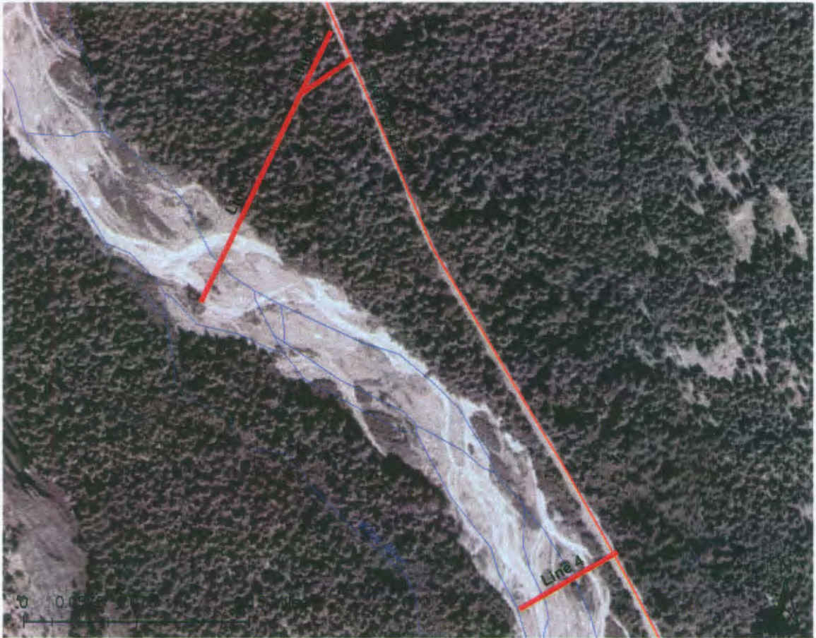
▲ FIGURE 1.11 Overview of cross sections along Highway 410 (White River). Line 1 has a bend; Line 1a is straight. River flow is from lower right to upper left.
