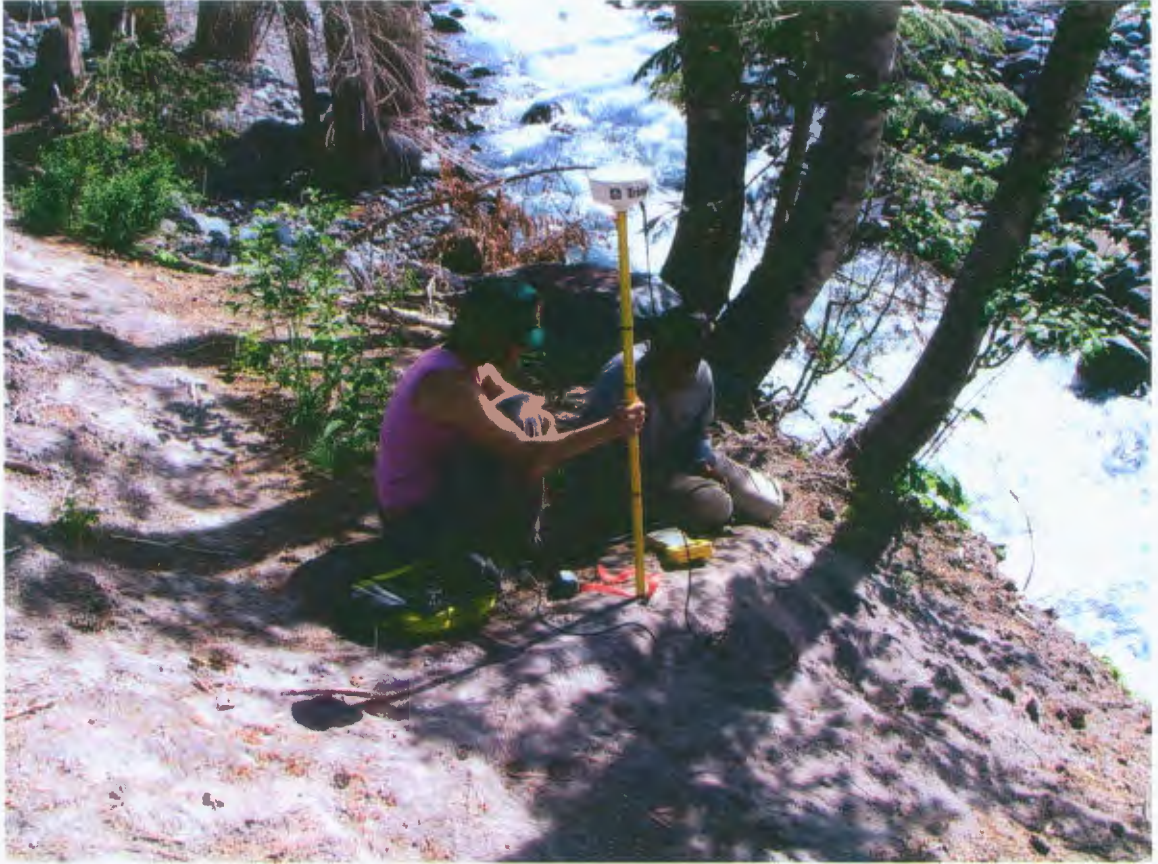
▲ FIGURE 3.3 Trimble Pathfinder Pro XR GPS shown mapping a control point (Photo: Scott Beason, 7/20/2006)
