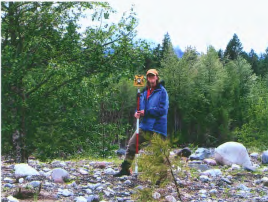
▲ FIGURE 3.2 Prism and adjustable-height rod assembly (Photo: Scott Beason, 6/17/2006).
