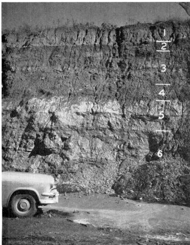
Figure 2. Typical sequence of coal overburden materials in a Marion County, Iowa highwall. From top to bottom are: (1) Wisconsin loess, (2) Kansan glacial till, (3) buff colored Pennsylvanian shale, (4) dark gray Pennsylvanian shale, (5) light gray Pennsylvanian shale and (6) gray Pennsylvanian shale grading into dark gray shale. The automobile is parked on the exposed 3 foot vein of coal.
