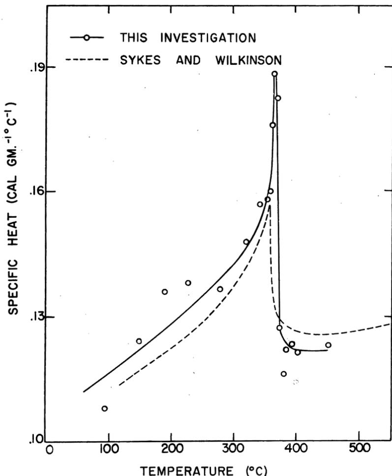
Figure 2. Specific Heat of Nickel.
