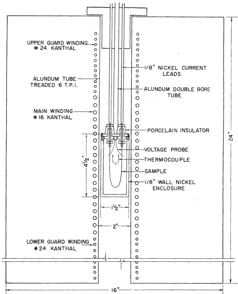
Figure 1. Furnace for the Measurement of Resistance Versus Temperature.
