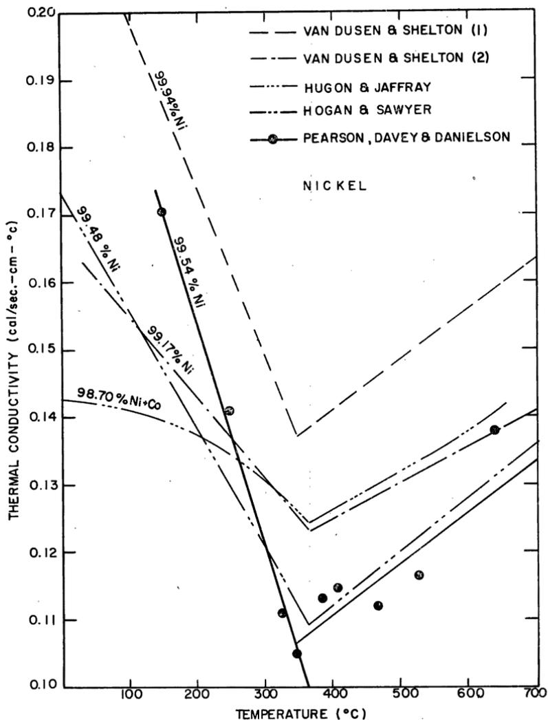
Figure 2. Thermal Conductivity of Commercial A Nickel.
