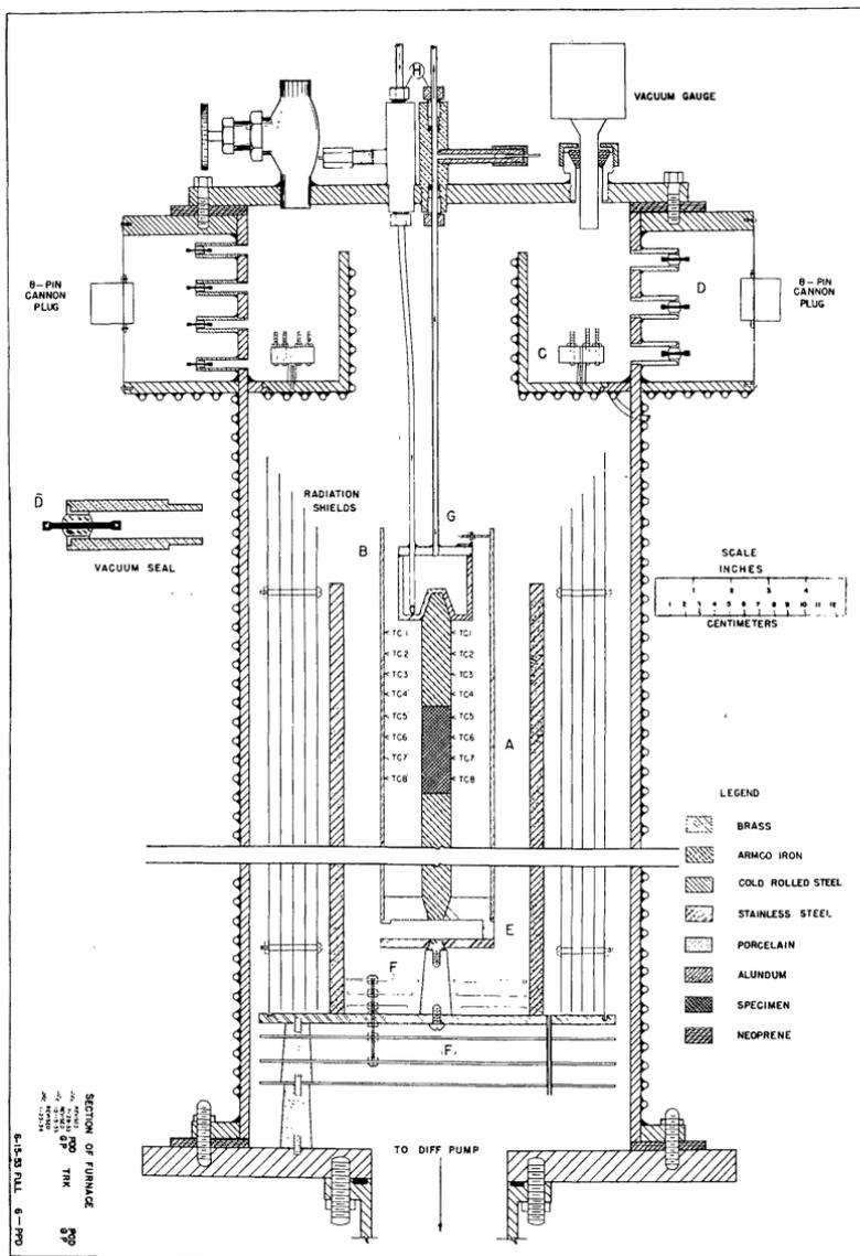
Figure 1. Vacuum Furnace for Thermal Conductivity Measurements.
