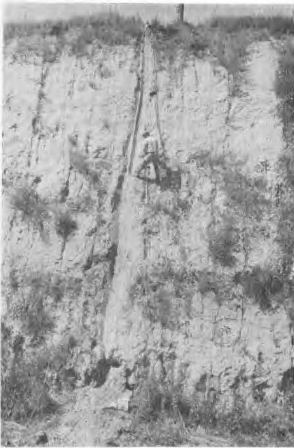
Figure 2A. Composite sampling by trenching and augering. Loess, section III, of Ida series.
