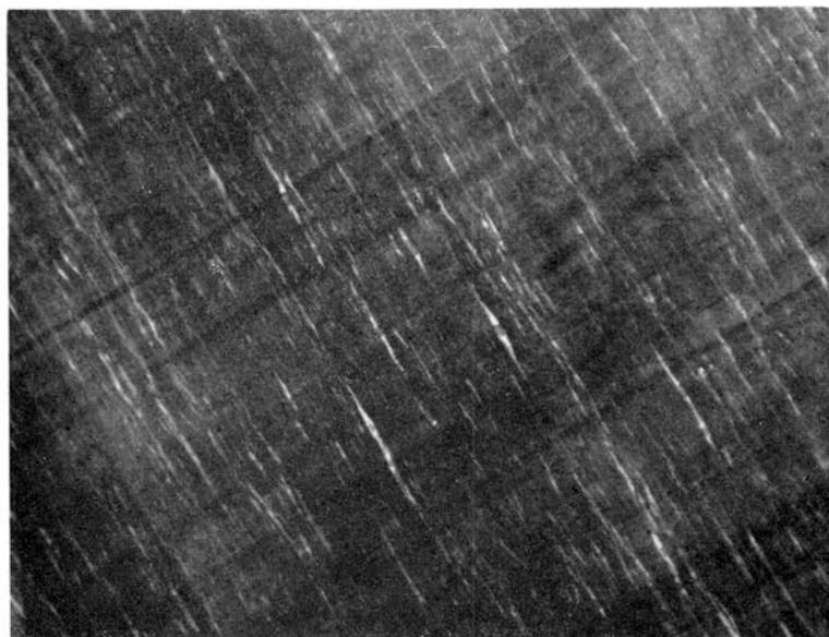
Figure 5. Microradiograph of a Leaded Steel. This steel is similar in composition to the steel in Figure 4 except that the sulfur content is below .05%. The lead is again noted to be associated with the non-metallic matter in the steel. The microradiograph was prepared by the same procedure as in Figure 4. The streaks running perpendicular to the rolling direction are caused by grinding roughness on the surface of the foil.
