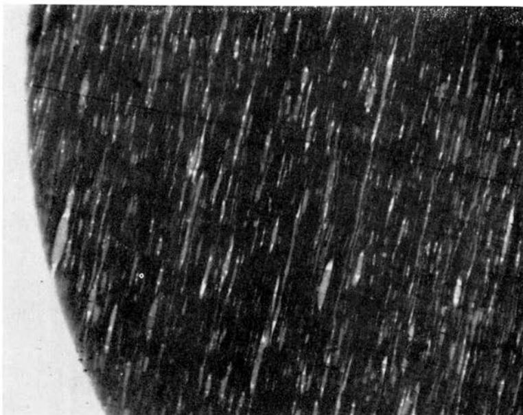
Figure 6. Microradiograph of a Leded High Sulfur Steel. This microradiograph, prepared with  $\text{CoK}\alpha$  radiation which falls on the short wavelength side of the absorption edge of manganese, includes the same inclusions examined in Figure 4. It is apparent that the centers of the inclusions are now lighter than the iron matrix. This results from using a radiation which falls on the top of the K-absorption edge of manganese, but not of iron. The centers therefore must contain manganese.
