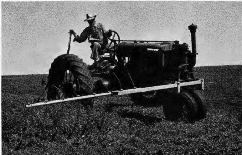
Figure 2. The "Ohio" type flushing bar was used in studies to find ways to reduce deaths of pheasant hens in hayfields.
