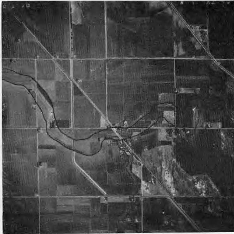
Figure 2. Geomorphic expression of the "flood basin" environment near Luton, Iowa. The only appreciable relief of this, that of an old channel of a small tributary stream which once flowed through the town of Luton.
