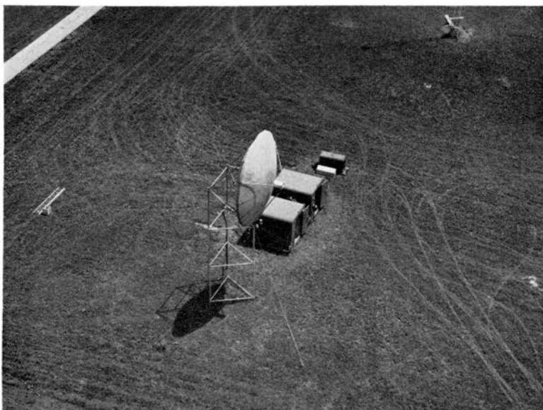
Figure 12. Typical air transportable duplex 1-kw scatter terminal designed for dual-diversity reception. One of two antennas is shown. Inflatable 15-foot paraboloid.
