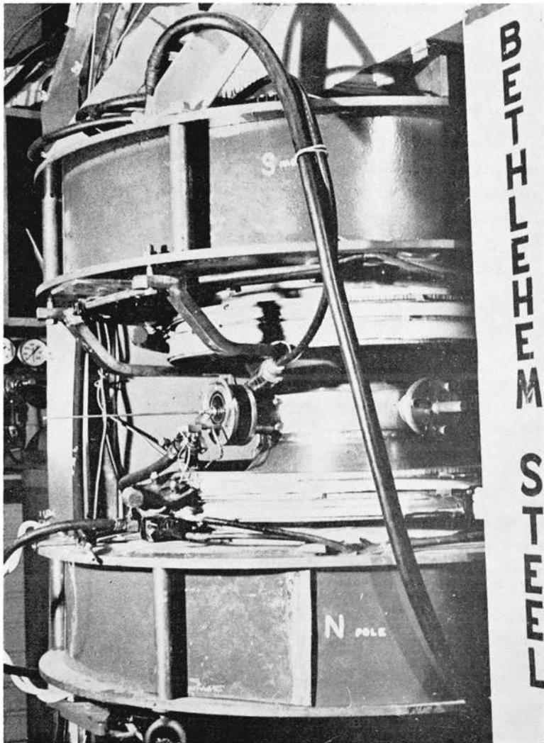
Figure 1. The Iowa State University cyclotron. The large cylinder-shaped objects marked "S" and "N" are the magnet coils. The magnet core, marked "Bethlehem Steel", is partially visible. The dee box is seen in the center of the photo between the tapered pole pieces of the magnet core. The distance from the top of the upper coil to the bottom of the lower coil is 25 inches.
