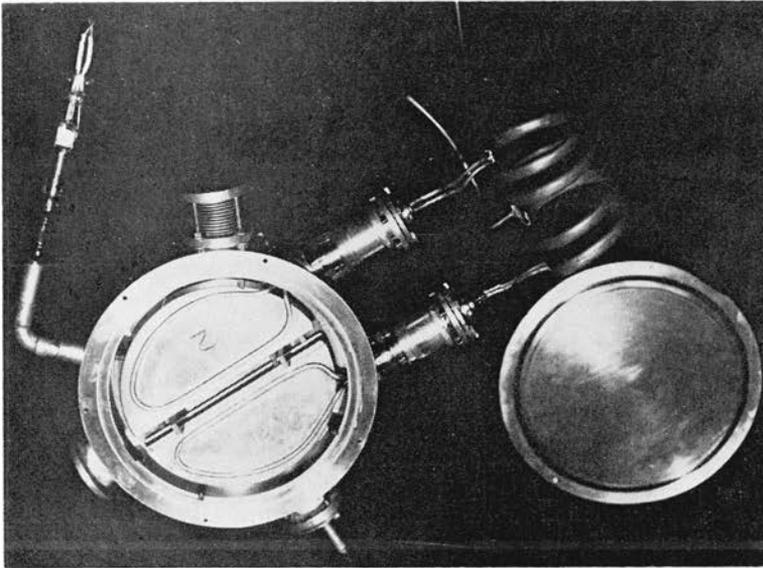
Figure 3. The dees box. The dees are the "D" shaped objects. The copper tubes that carry cooling water are seen near the edge of each dee. The copper helix on the right is the coil of the radio frequency tank circuit. The lid of the dees box is seen at the lower right. The bakelite spacers between the dees are for jiggling purposes only and are removed when the machine is in operation.
