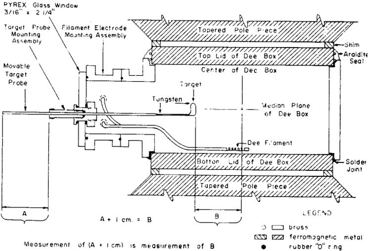
Figure 5. A cross-section of the dee box illustrating the relative positions of the target and the ion source within the box. It also shows the taper, shoulder, and shims of the magnet poles (from Crosland).
