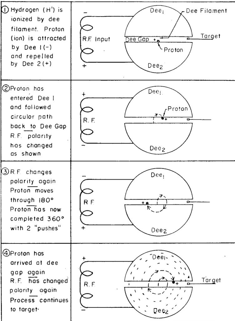
Figure 2. A schematic view of the dees showing the path of the accelerated proton. The magnetic field is perpendicular to the plane of the dees (from Crosland).
