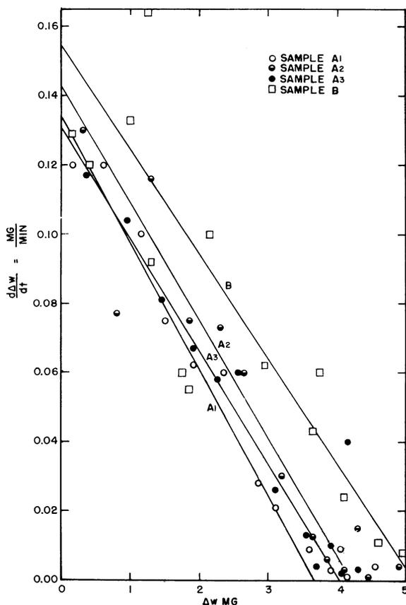
Figure 2. Differential plot of weight gain by platinum oxide on exposure to air.
