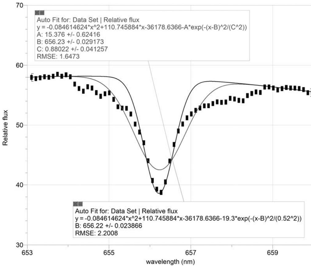
Fig. 8. Gaussian curve-fits of the H-alpha absorption during the secondary eclipse, when the primary component dominates the spectrum (phase 0.525).
