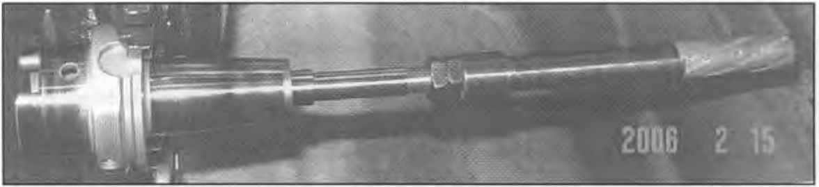
Figure 9. Example of a super abrasive tool used in machining center.
