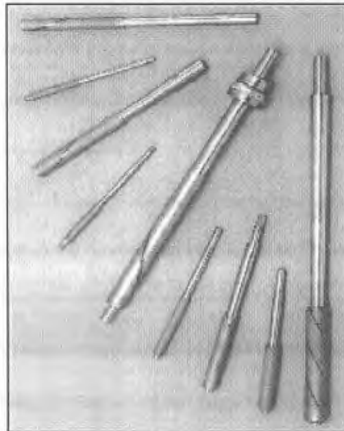
Figure 8. Examples of super abrasive tools (Arunachalam & Rajendran, 2005).
