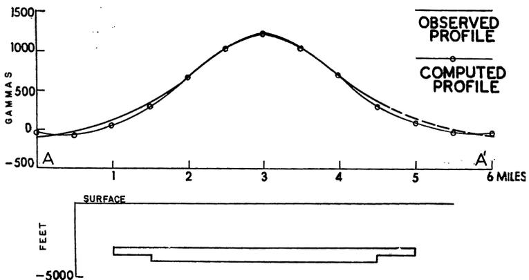
Figure 3. Observed and computed magnetic profiles over assumed body.
