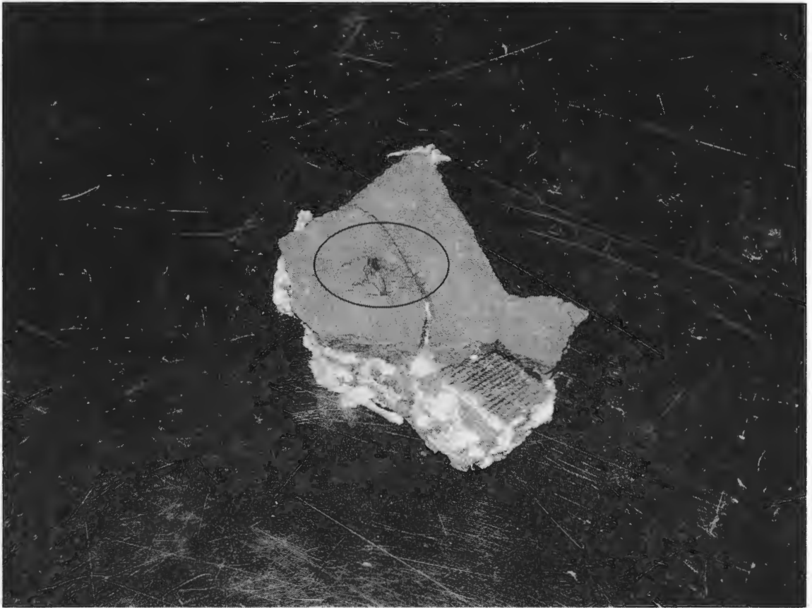
Figure 4 Photo of heat focused pocket formation.
