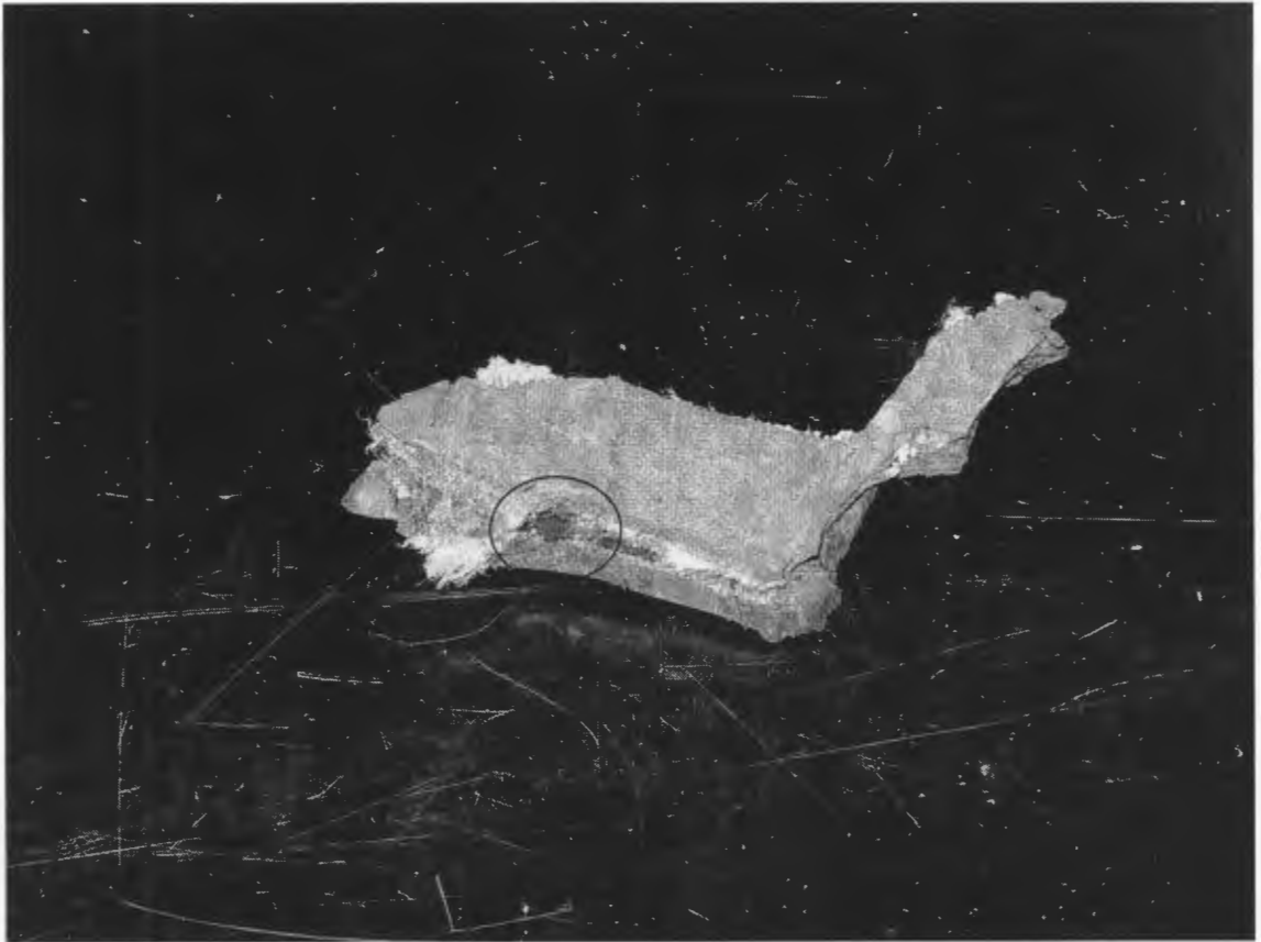
Figure 6 Photo of a microwave energy focused heat pocket.
