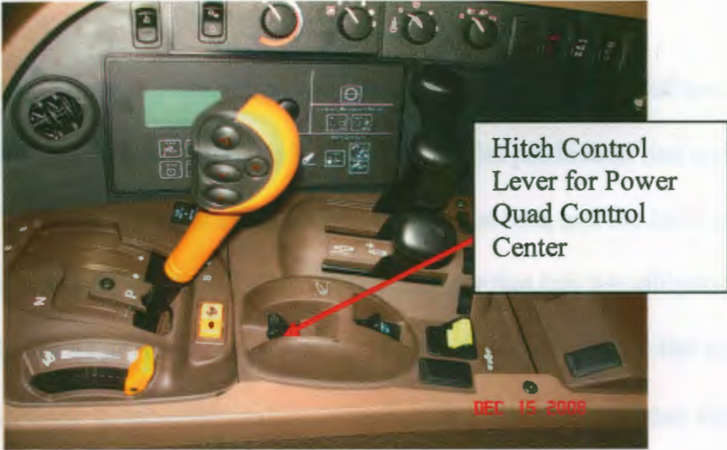
Figure 13a. Power Quad Transmission (PTQ) Control center
