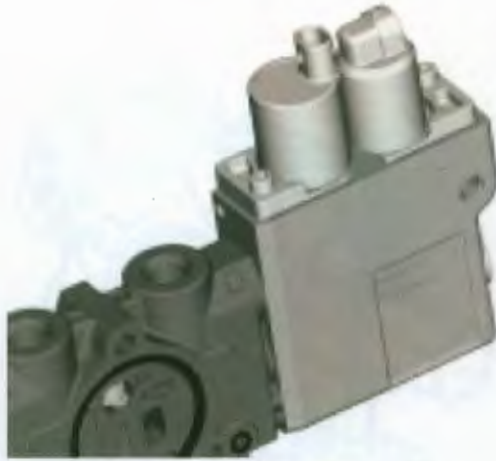
Figure 7b. Hitch control valve (Electrohydraulic actuator).
