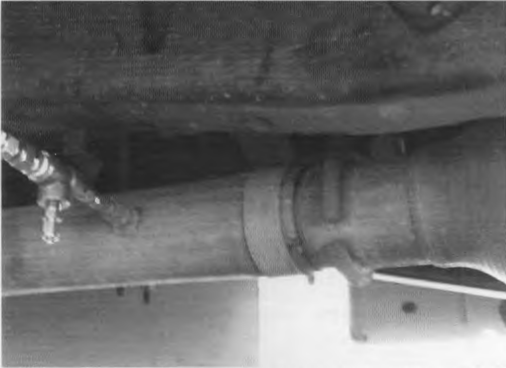
Figure 9. After the DPF measurement of PM mass concentration setup for the DPF filtration efficiency study.
