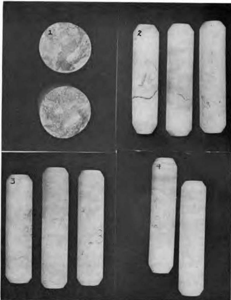
Figure 1. Fracture surfaces of broken styolitic seam of core number 16. This core fractured under its own weight when it was removed from sodium hydroxide.
