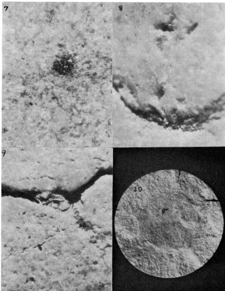
Figure 7. Clustering in the pyrite distribution. Small particles are shown in the opaque cluster as well as numerous single particles.
