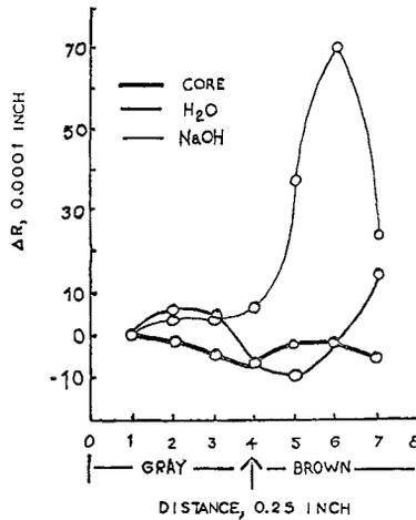
Figure 5. Axial distribution of radial expansion. Curves for untreated and autoclave treated cores from the same rock are presented with the change from gray to brown color to show the dependence of the magnitude of expansion on color.
