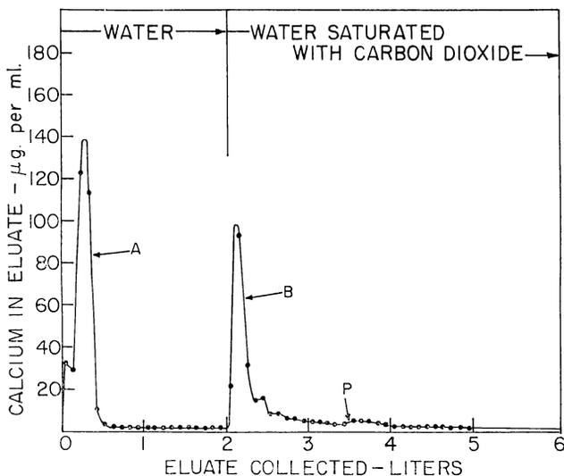
Figure 1. Adsorption and elution of calcium on Tensleep sandstone. A. Excess calcium passing through column; B. Adsorbed calcium eluted by water saturated with carbon dioxide; p. Elution stopped for 13 hours
