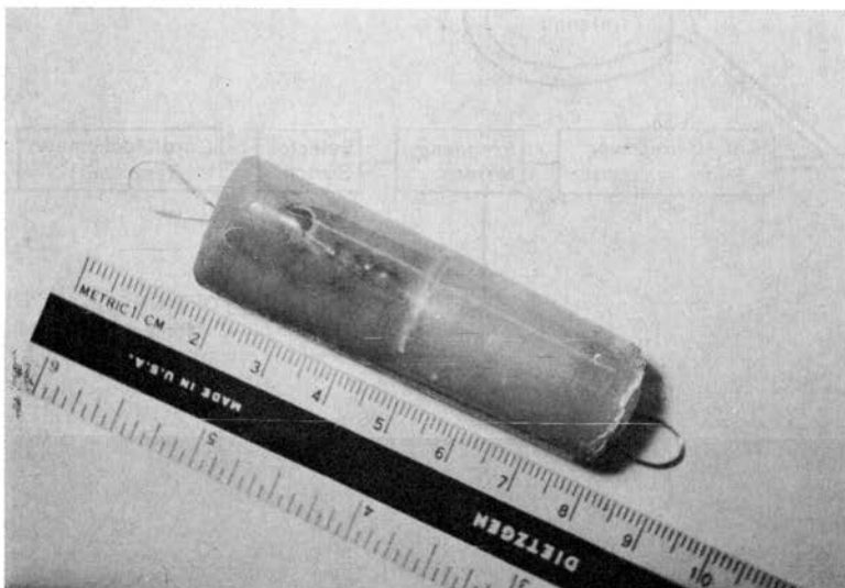
Fig. 4. View of typical implantable Iowa radio transmitter for recording heart rate and EKG.
