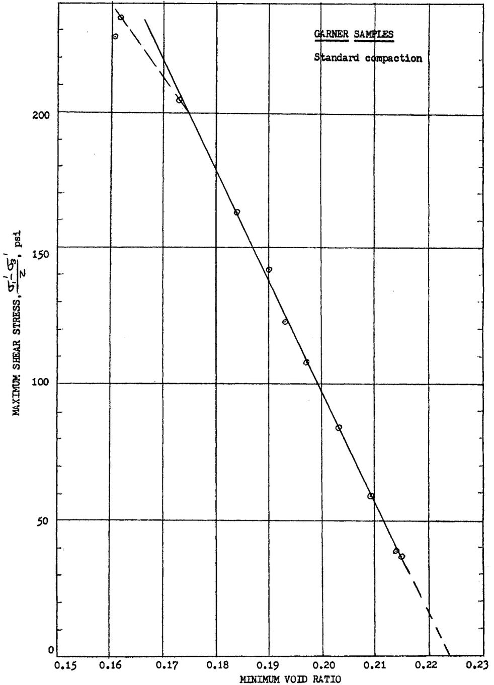
Figure 5. Garner Stone: maximum shear stress as related to minimum void ratio
