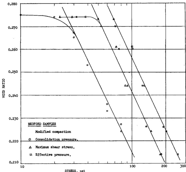
Figure 2. Bedford stone. consolidation pressure, maximum shear stress, and effective normal pressure as related to void ratio.
