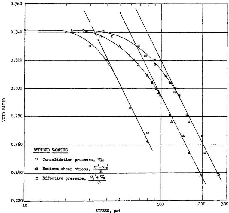
Figure 1. Bedford stone: consolidation pressure, maximum shear stress, and effective normal pressure as related to void ratio.
