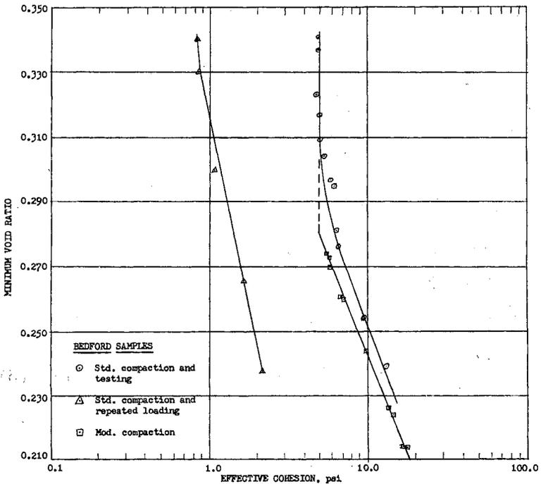
Figure 4. Bedford stone: relationship between the minimum void ratio and the effective cohesion.
