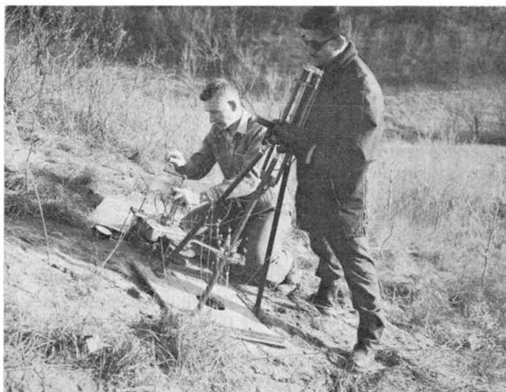
Figure 2. Field set-up for shear test.
