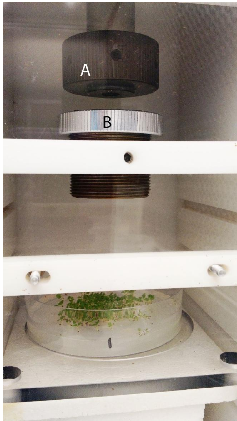
Figure 8: Positioning of Arabidopsis thaliana Columbia in the biolistics chamber. A: Location of rupture disc at the end of the helium acceleration tube. B: Location of microcarrier screen, microcarriers coated with DNA solution, and stopping screen. Seedlings sit 80 mm below the stopping screen within the chamber with no barriers between.
