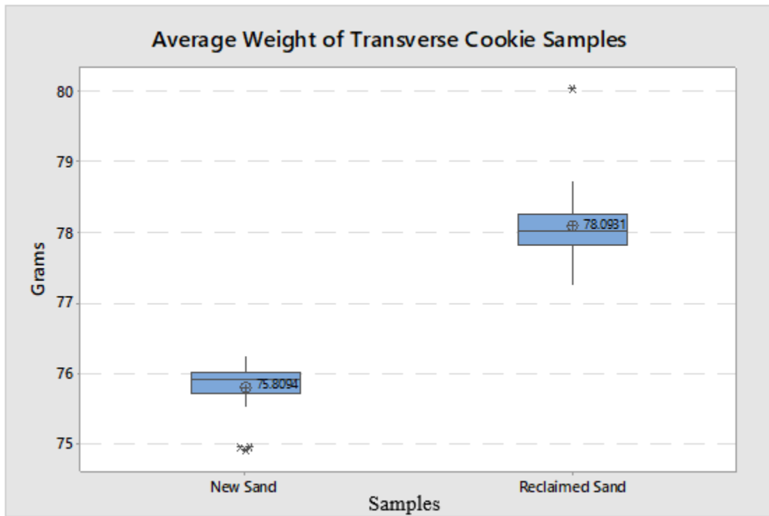
Figure 24 Measured weight of the transverse cookie samples. Weights represent the group of all three samples together.
