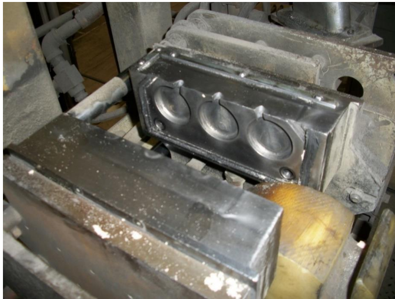
Figure 8 Transverse Tensile Cold Box Core Mold, John Deere Foundry
