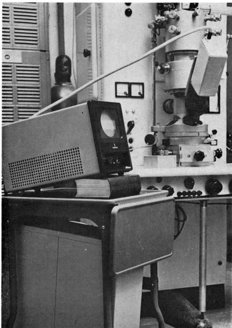
Fig. 2. Small box on microscope table has intensity and contrast controls for the wall-mounted monitor. Control monitor in foreground has its own controls. Control unit is visible under the monitor.
