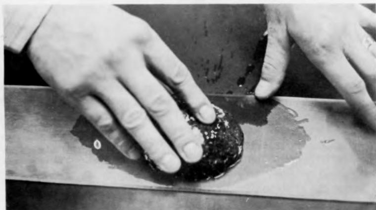
Fig. 3. A paste of carborundum powder is placed on a glass plate and the coal slab is rubbed until smooth.
