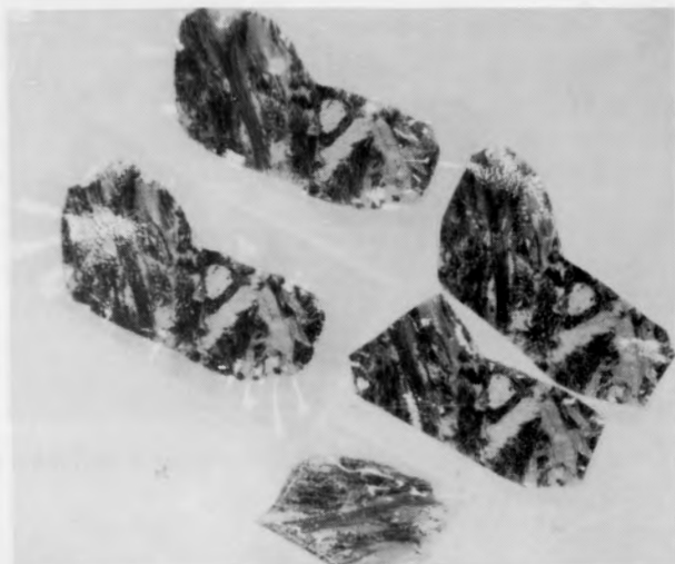
Fig. 6. Several peels taken from a single slab and mounted on cardboard sheets.
