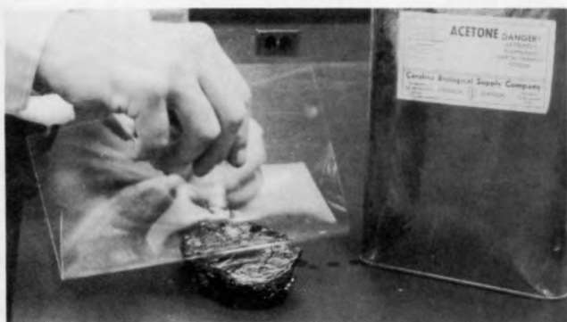
Fig. 5. A cellulose acetate sheet rolled onto a slab. Only half of the slab is covered with acetone as the rolling action of the sheet will serve to spread the acetone over the slab.
