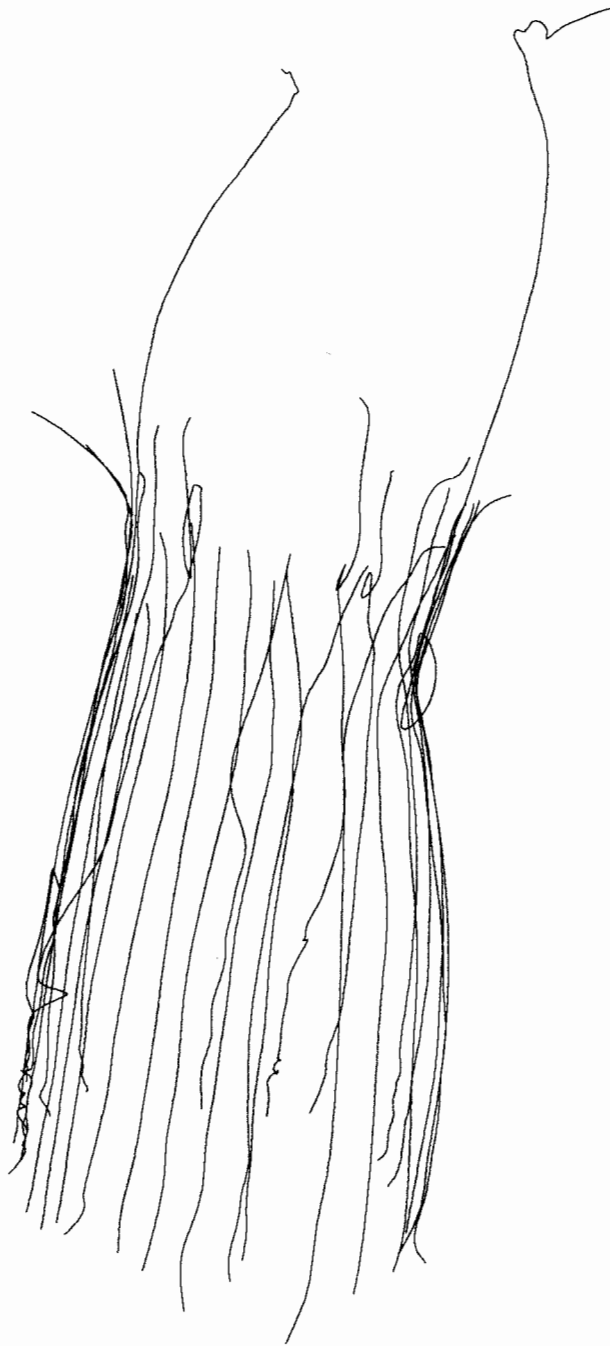
Figure 12. The digitizer data prepared for analysis. Hard returns were added to the end of each record, positive Y values were changed to negative Y values, and points recorded in the reverse X direction between line segments were removed.
