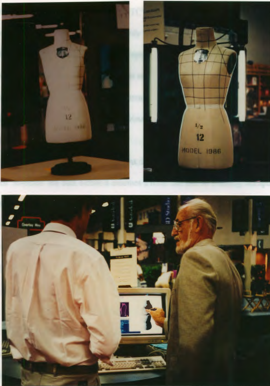
Figure 5. A laser scanner by Cyberware is used to measure a one-half-size dress form at SIGGRAPH. In the top two photos, the scanner circled around the dress form. In the bottom photo, the data, wireframe, and color surface is viewed in the computer monitor.
