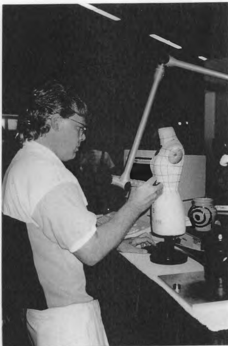
Figure 4. A mechanical digitizer by FARO is used to measure a one-half-size dress form at SIGGRAPH.
