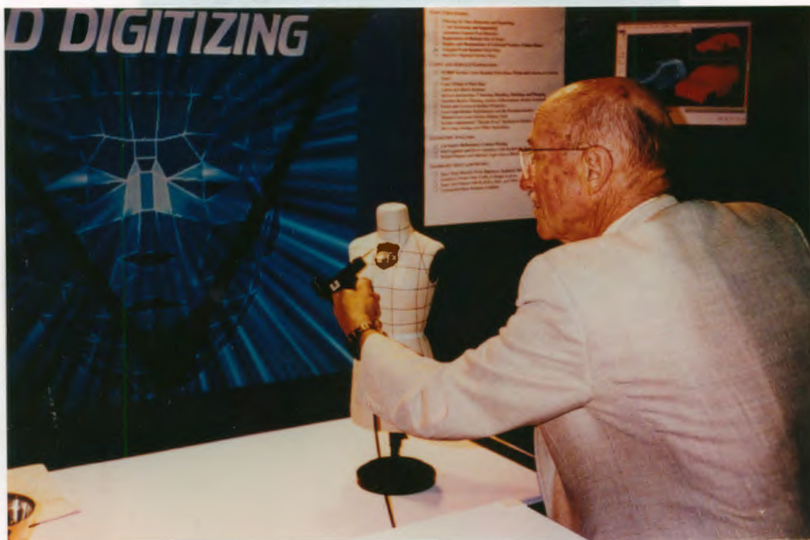
Figure 3. A sonic digitizer by Science Accessories Corporation is used to measure a one-half-size dress form at SIGGRAPH. Note the triangular microphone frame on the wall.
