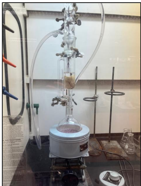
Figure 1. Soxhlet extraction set up.
