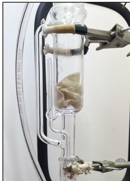
Figure 2. Close up of Soxhlet extraction set up.
