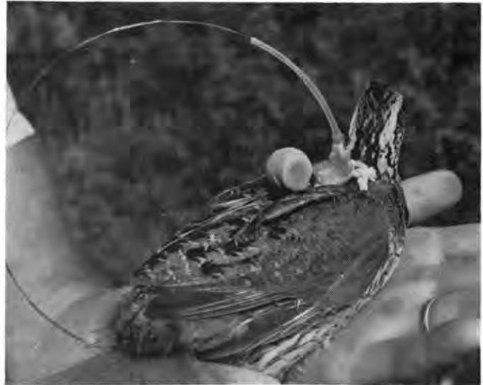
Figure 1. Transmitter and battery.
