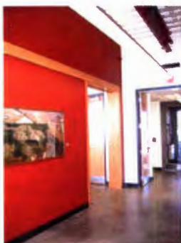
This hallway connects the north side of the building to the south side without passing through the classrooms. This also helps to act as sound control when the classrooms close their doors to the hallway, the dead space between helps to absorb the sound.
