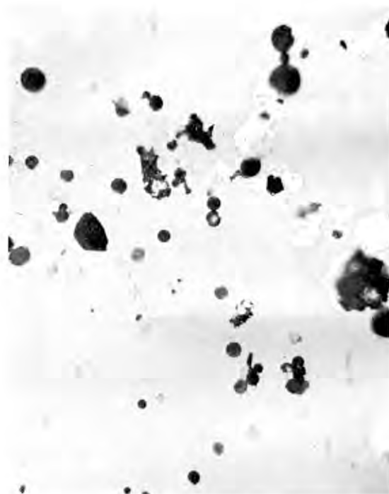
Figure 1. Photomicrograph of fly ash sample C-1 (whole sample) at 250x. There is an abundance of spherical and irregularly-shaped clear and dark particles.
